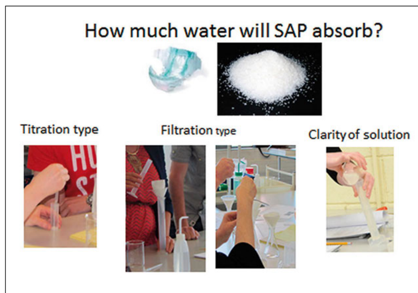
Figure 3. Approaches taken to determine the amount of water absorbed by SAP.
